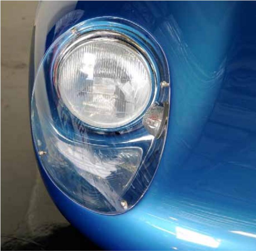
Headlights are recessed into the body and covered with a removable shield for protection and easy maintenance.
