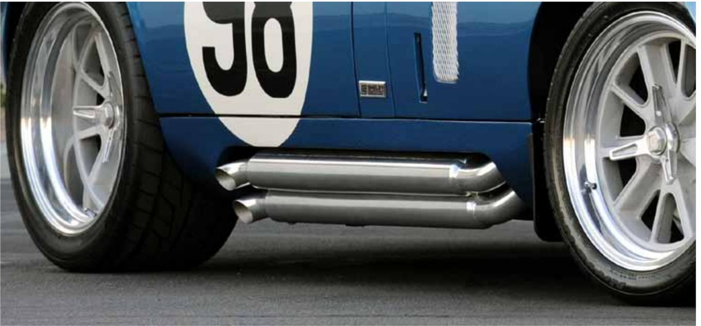
Side pipes and headers are standard with every Daytona Coupe. Primered is no charge. However, we do offer silver ceramic coated and black ceramic coated pipes at a nominal up charge.
